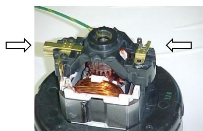
Fig 2: 1 Motor Brush Removed
